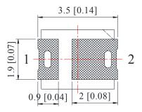
**Recommended Soldering Pad Dimensions**
