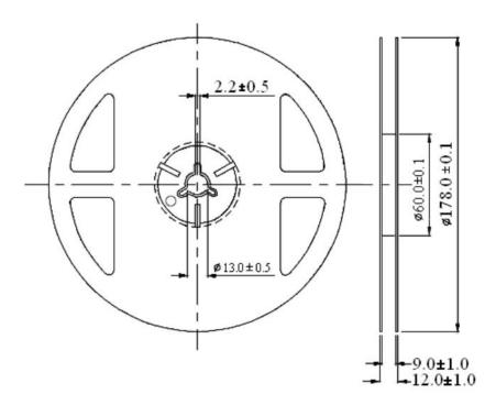
Unit: mm Tolerance:  $\pm 0.25$ mm
